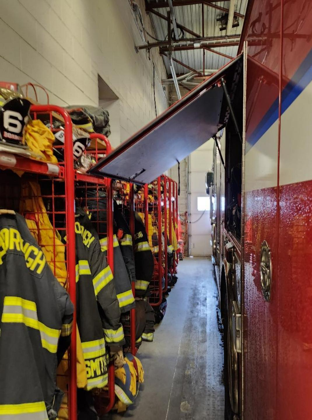
The firehouse apparatus bay is so cramped that access to the vehicle equipment storage hatch cannot be opened fully
